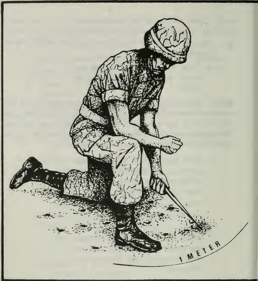
Figure 228. Probing for magnetically fuzed mines.
